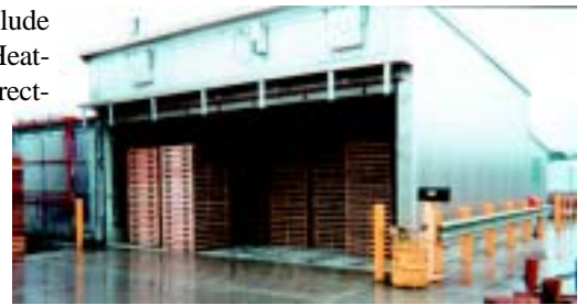
SII Dry Kilns Heat Treater system for pallets.
