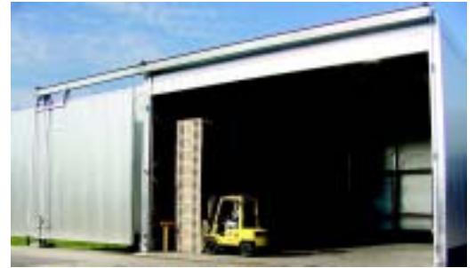
Brunner-Hildebrand pallet heat treating chamber at Acme Skid & Plug division of Apache Products in Silsbee, Tex.
